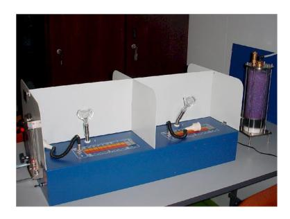
The Mannebeck TO7 dynamic olfactometer was used, with four stations, which uses a panel of four people to send a "dirty" air mixture in order to determine the "smell" level of a "dirty" air sample. and "clean air with increasing concentrations until the smell is perceived. The measurement ends when all panelists perceive the smell.
